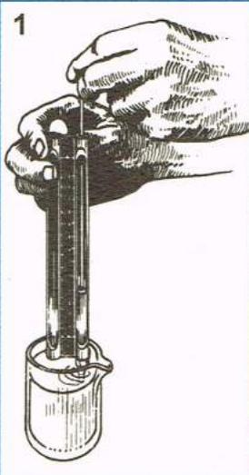
Place a small quantity of oil into a container (Fig. 1), then insert nozzle of VISGAGE into this oil (fluid) when temperature is approximately 27°C (80°F).
